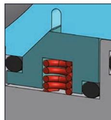
**2. Spring loaded sealing system**
