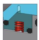
**3. Spring loaded sealing system** Guarantees almost same torque at different temperatures
