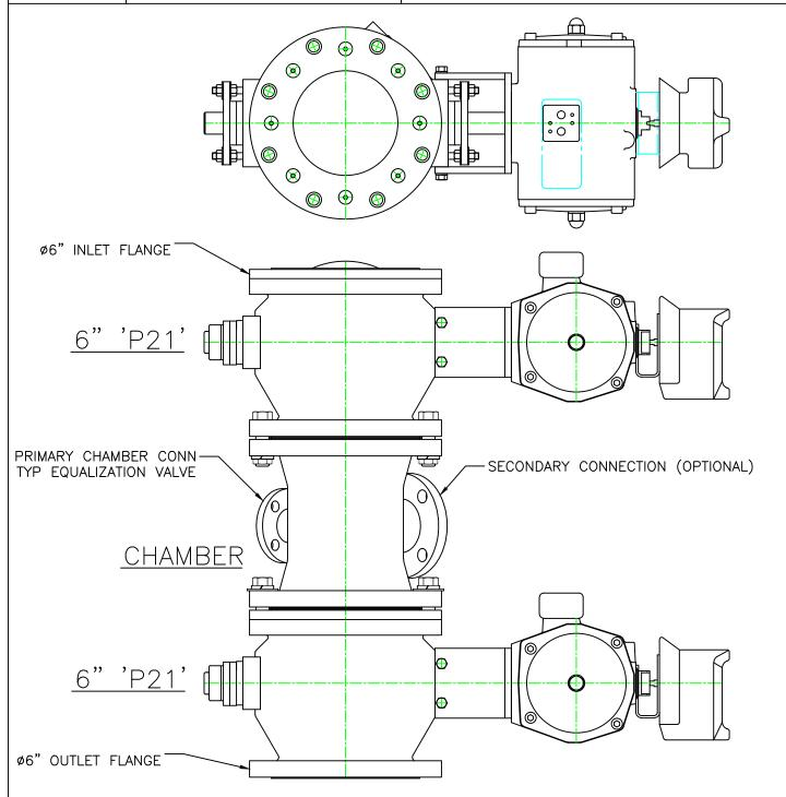
VALVE SIZES, CHAMBER SHAPE AND SIZING, VALVE ORIENTATION, AND ADDED OPTIONS ARE BASED ON CUSTOMER SPECIFICATIONS. SEE OTHER AIRLOCK DRAWINGS FOR EXAMPLES OF FLIPPED OUTLET VALVES, CHAMBERLESS "DOUBLE DUMP" AIRLOCKS, ETC.
