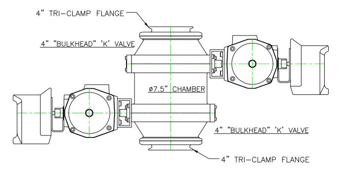
VALVE SIZES, CHAMBER SHAPE AND SIZING, VALVE ORIENTATION, AND ADDED OPTIONS ARE BASED ON CUSTOMER SPECIFICATIONS. SEE OTHER AIRLOCK DRAWINGS FOR EXAMPLES OF UNFLIPPED OUTLET VALVES, CHAMBERLESS AIRLOCKS, ETC.
